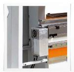
CNC Motorised Crowning System (O) CNC crowing system that communicates with the CNC controller, performs crowning automatically and enables the part to be at even bending angle at any given point.
