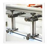
Backgauge Fingers (O) Specifically designed folding backgauge fingers.
